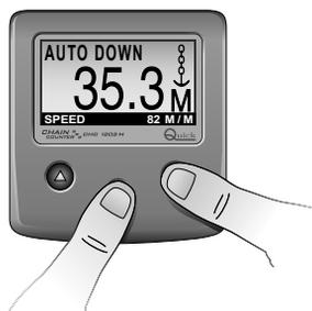
The automatic lowering procedure can be interrupted by pressing any key of the chain counter from which the procedure was activated, by activating the up function from an external device (from another chain counter or other control) or by shutting off the chain counter.
