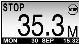
The date and time are stored even when the chain counter is shut off (it is equipped with a buffer battery).
