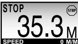
The precision of the chain speed reading is  $\pm 1\%$  accurate.
