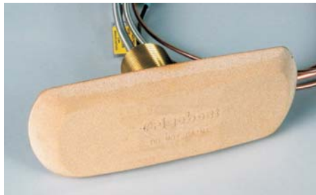
THE KEEL COOLER IS MANUFACTURED FROM MARINE GRADE BRONZE WITH CUPRO-NIKEL PIPING.
