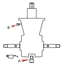
Check the oil in the leg annually. Change if necessary: oil drain plug under the anode (A). Oil level screw on the side of the leg (B). Copper washer should be changed. The anode should be checked frequently and changed if necessary (at least once a year). If you find water in the oil, it is necessary to change the propeller shaft oil seals. The anode must be checked frequently and changed if necessary (at least once a year).
