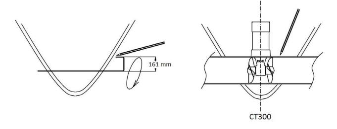
Replace the tunnel. To secure its position apply reinforced fibreglass filler to all areas, both inside and out, taking care to entirely fill the space between the hull and the tunnel. Laminate using a minimum of 8 layers of **ISOPHTALIC RESIN** alternated with mat and roving.
