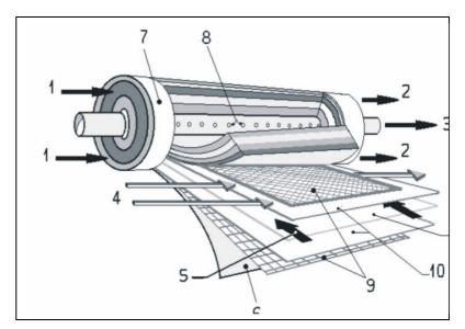
The **semipermeable membranes**, used in the production of BAITEK Watermakers, are constructed in synthetic material with spiral structure and packed in very distinguished packaging, called **modules**. The membranes, suited for desalinate sea-water, have a salt reaction of beyond 99% and can operate until 40°C water temperature.
