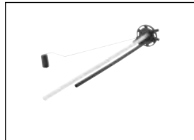
Adjustable ALAS II lever-arm sender
