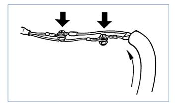
Slide the heat shrink tubing over the cable connections and then heat with a hot-air fan over the entire length until it shrinks.
