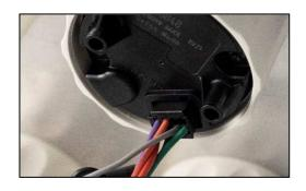
Use the 2-pole connector to connect the external pushbutton.
