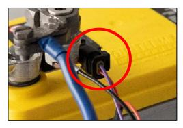
Connect the resistive level sensor plug (AMP SuperSeal 1.5 series 2 Pin) to the Level Sensor if there is one in your system.
