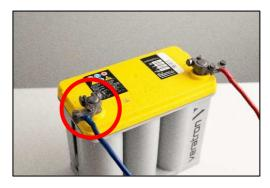
Mount the wire harness' ground cable on the IBS ground bolt. Use the battery pole adapter to fasten the dedicated ring-type connector.
