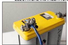
Connect the Hirschmann plug next to the black ring-type connector (2 poles for 12V-Variant/ 3 poles for 24V) to the battery sensor.
