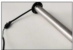
Connect the VL Flex 52 connector (Tyco / Hirschmann 8 pole MQS plug) to the instrument.
