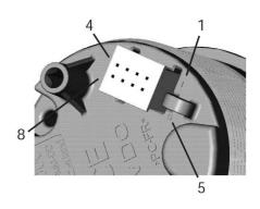
Instrument rear view Tyco / Hirschmann 8 pole MQS plug
