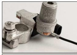
Now mount the system ground cable (the one that has been attached directly to the battery before) onto the battery pole adapter on the IBS.
