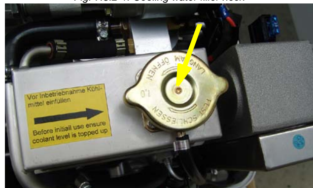
Fig. 7.5.2-1: Cooling water filler neck
