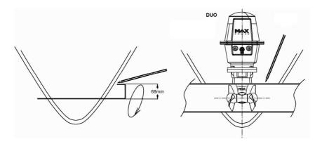
Replace the tunnel. To secure its position apply reinforced fibreglass filler to all areas, both inside and out, taking care to entirely fill the space between the hull and the tunnel. Laminate using a minimum of 8 layers of **ISOPHTALIC RESIN** alternated with mat and roving.
