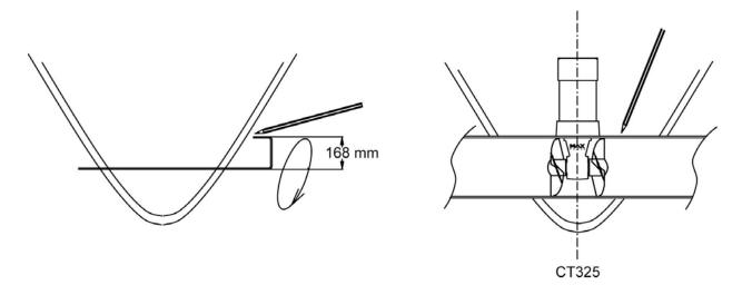
Replace the tunnel. To secure its position apply reinforced fibreglass filler to all areas, both inside and out, taking care to entirely fill the space between the hull and the tunnel. Laminate using a minimum of 8 layers of **ISOPHTALIC RESIN** alternated with mat and roving.
