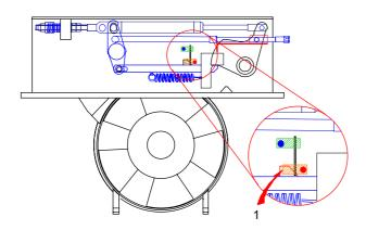
The proximity switches on the thruster indicate to the control box in witch position the thruster is in.
