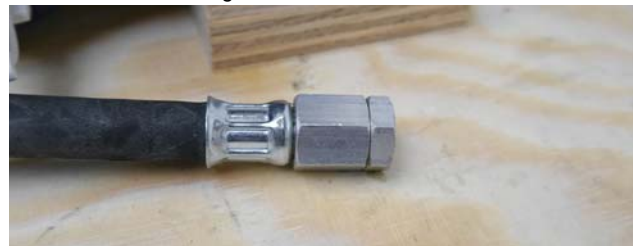
Fig. 6.8-2: Oil drain hose
