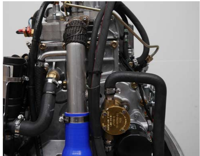
Fig. 6.13.3-3: Raw water pump
