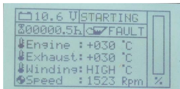
Fig. 16.1.1-2: Warning: „Winding temperature too high“
