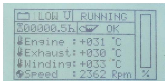
Fig. 16.1.1-1: Warning: „Battery power too low“
