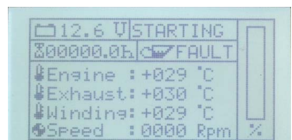
Fig. 12.3.3.2-2: Default display screen during start-up
