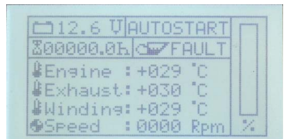
Fig. 12.3.3.7-1: Default display screen in autostart mode
