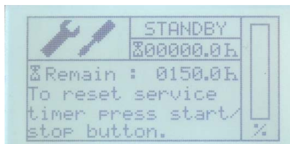
Fig. 12.4.7-1: Resetting the time until the next service
