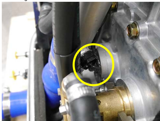
Fig. 6.2.6-2: Thermo-switch at exhaust connection
