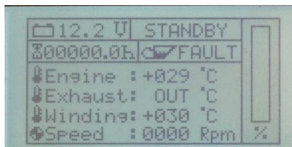
Fig. 16.2-2: Fault: „STARTING FAILS“, start-up process was not successful
