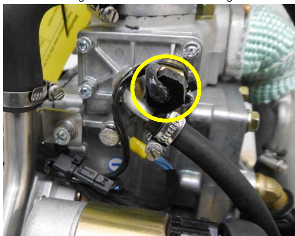
Fig. 6.2.6-1: Thermo.sensor at engine
