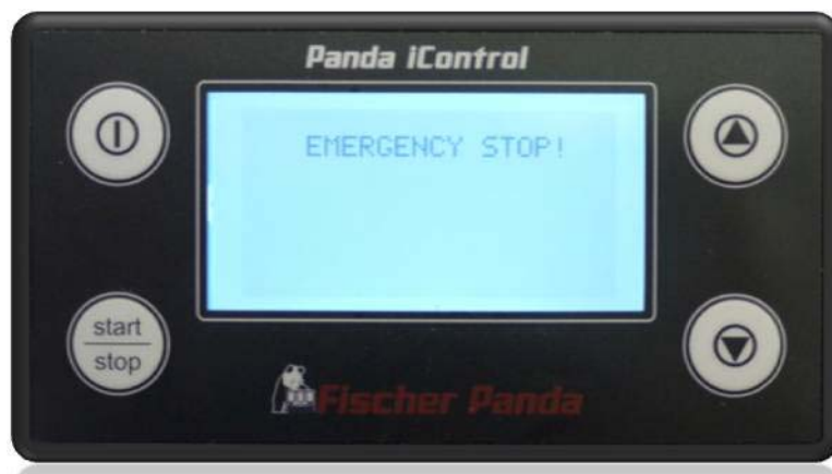
Fig. 12.5-2: Panel shows Emergency Stop
