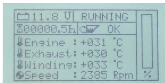
Fig. 12.3.3.4-1: Default display screen in operation mode
