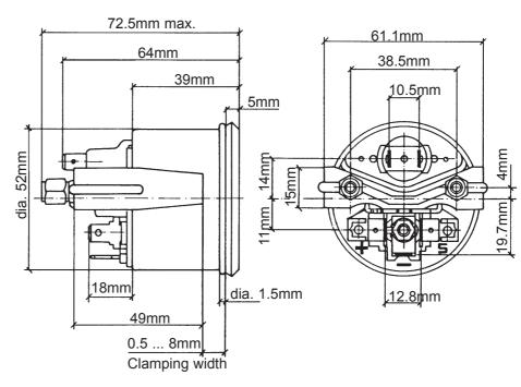
Pin assignment: Pin +: + 12 V or + 24 V terminal 15 Pin -: Ground, terminal 31
