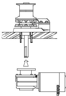
Join the under deck part to the top part inserting the key (224) of the main shaft into the key way of the gearbox. Tight the nuts on the studs. Join the cables to the electric motor. Introduce the rope/chain into the gipsy , operate the "UP" switch of the foot switch or remote control and the chain will automatically be fed into your locker. Take care to keep hands and feet well clear of incoming chain. If the windlass runs in wrong direction , change over M1 and M2 cables at the control box.
