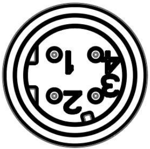
M12 4-poles Code D connector, display pin view
