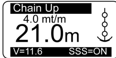
In order to activate or deactivate SSS mode, it is necessary to enter the main menu pressing the button Enter for at least 3 seconds and select the "Sec Sail System" menu.
