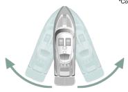
Activating both bow and stern thruster to push the boat sideways
