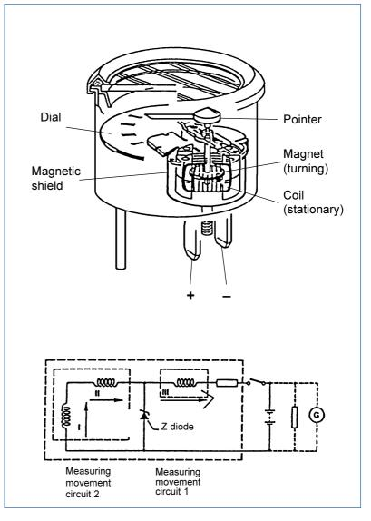
measuring circuit 1 containing coil III increases with the measured voltage, whereas it remains constant in measuring circuit 2 with coilsi and II. The turning magnet carrying the pointer follows the direction of the field resulting from measuring circuits 1 and 2, thereby indicating the measured voltage.
