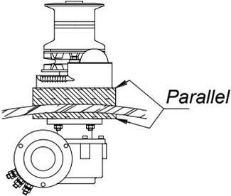
The PROGRESS TWO models are made by a top part , including drum, gipsy and base , and an under deck part , the gearbox and electric motor.
