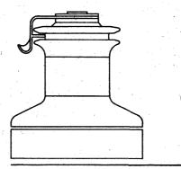
Routine Maintenance No. 65 ST A Release four allen screws (46) and remove top cap (1). B Remove split collets (45). C Lift off stripper arm (44). D Remove flanged bush (43). E Lift drum assembly (7) off centre stem assembly (9). F Remove bearings (10) and thrust bearing (41). G Clean thoroughly all parts using kerosene (paraffin) or white spirit. Dry with a nonfluffy cloth. H Replace thrust bearing (41) and bearings (10) on centre stem (9)
