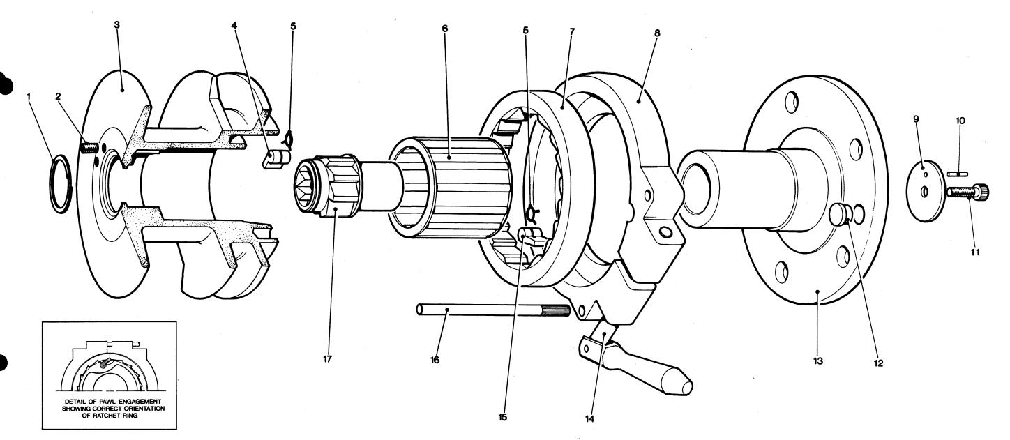
Maintenance No 1 — Mark I A Remove halliard wire from drum (3) by releasing grub screws (2).
