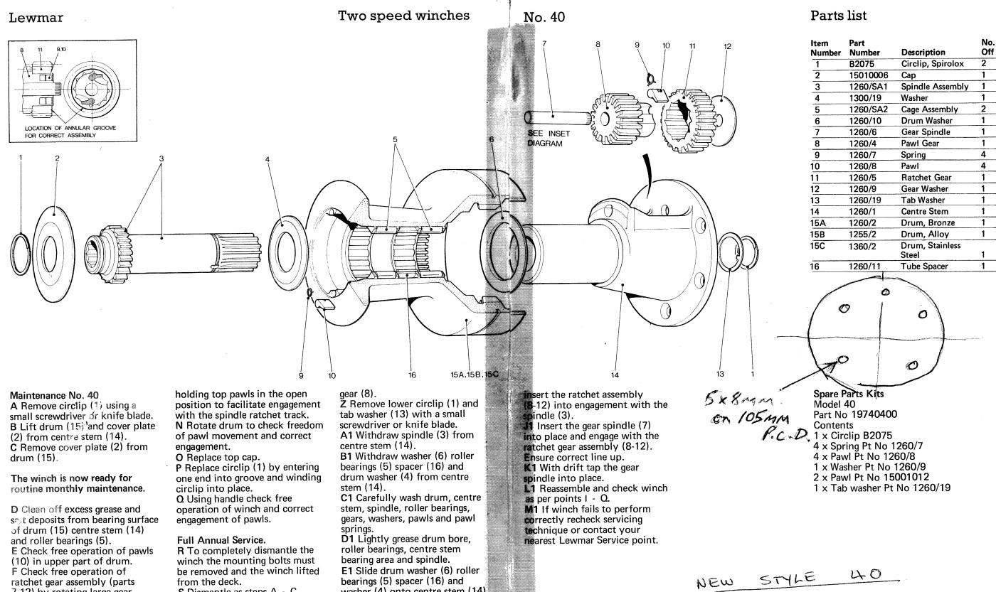
7-12) by rotating large gear. S Dismantle as steps A - C. T Remove two pawls (10) and G Check free rotation of spindle two pawl springs (9) from drum. (3) in centre stem (14). H If satisfactory proceed with U Support the centre stem assembly (14) on its base on a routine maintenance. If not firm structure (work bench etc.). continue to Full Annual Ensure the lower exit of bearing Service.
