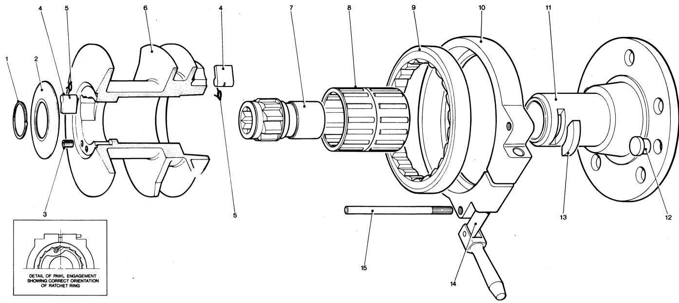
Maintenance No 1 — Mark II A Remove halliard wire from drum (6) by releasing grub screws (3).
