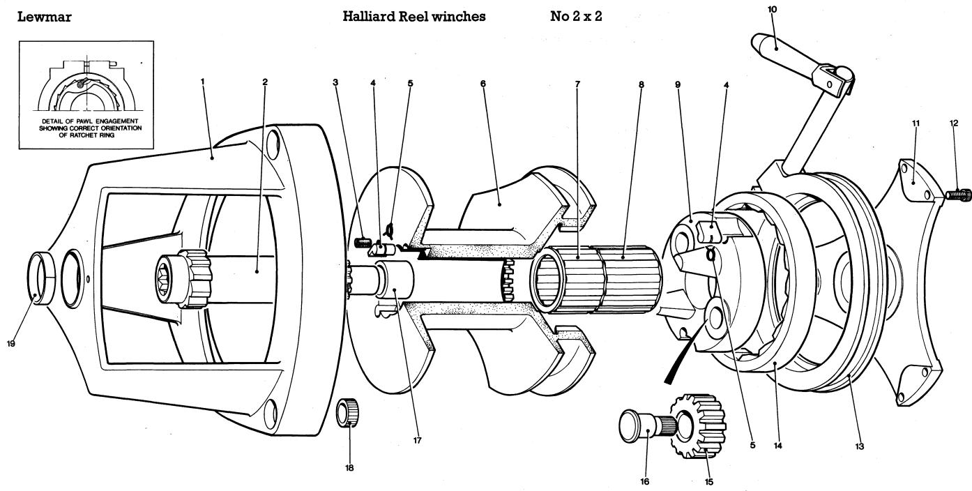
Maintenance No. 2 x 2 A Remove halliard wire from drum (6) by releasing grub screws (3) and remove winch
